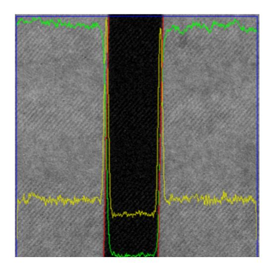
LEDs 25cm behind the diffuser, 500ms exposure time required.
