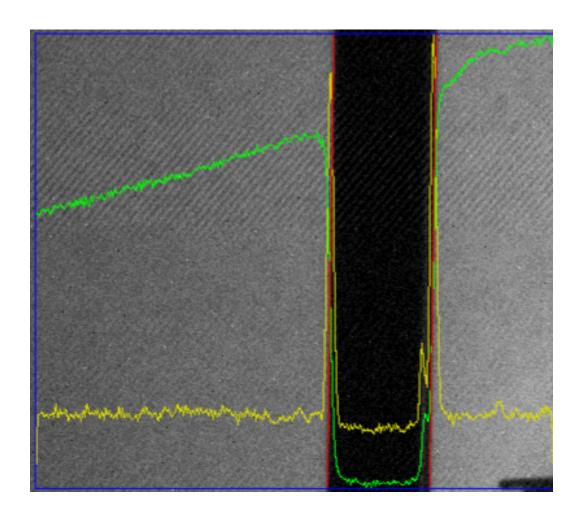
Same setup, except this time the LEDs and the object are both 30cm from the diffuser. 200ms exposure time is required to find the object's edges.
