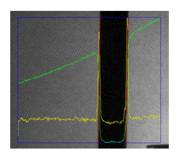
Optical Post is 20 cm from diffuser, as is the LED array. The LED array shines light on the diffuser at a 45 degree angle off to the right of the image.
