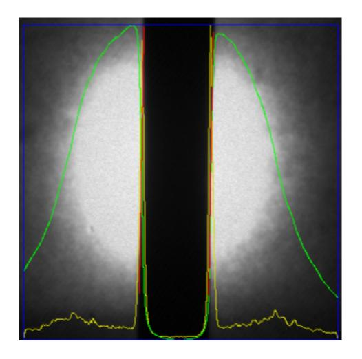
LEDs 2cm behind the diffuser, 500ms exposure time required.
