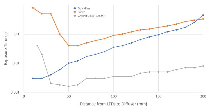
We vary the distance from the LEDs to the diffuser, using both a paper and opal glass diffuser to determine what position gives the sharpest silhouette. The y-axis is the minimum exposure time required for the analysis to find both the left and right edge fully.
