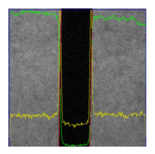
LEDs 15cm behind the diffuser, 200ms exposure time required.
