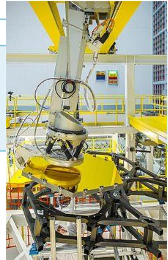
Robotic arm installing mirror segments for the James Webb Space Telescope - NASA
