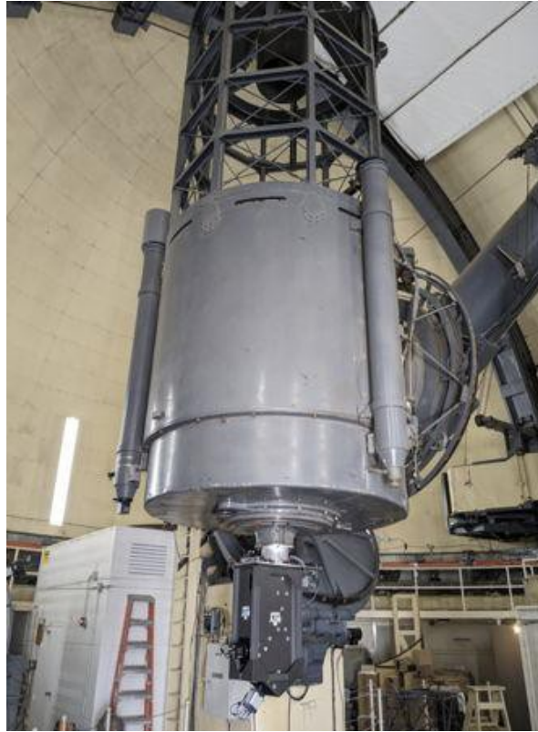
Figure 10: The Otto Struve Telescope and Dome. An astronomical instrument is installed at the Cassegrain viewport, in the same location we plan to install the DFPS-A80.
