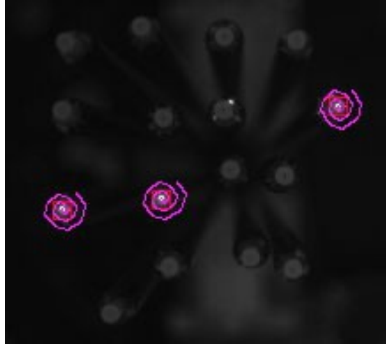
Figure 3: DFPS-A16A Fiber Tips Seen in Fiber View Camera. Three are executing spiral reset, their movement traced by magenta lines.
