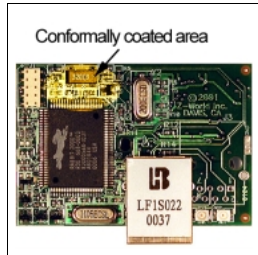
Figure A-4: RabbitCore RCM2200 Areas Receiving Conformal Coating
